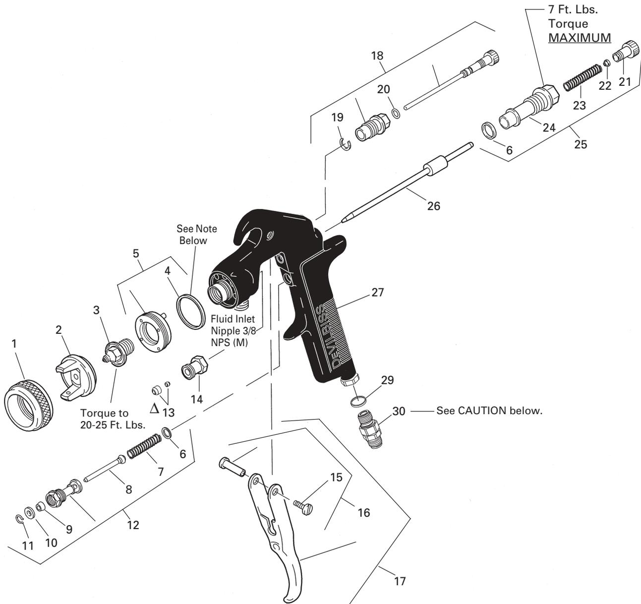
△ Detail Ref. No. 13 - Two piece packing covered by U.S. Patent No. 5,209,501.
