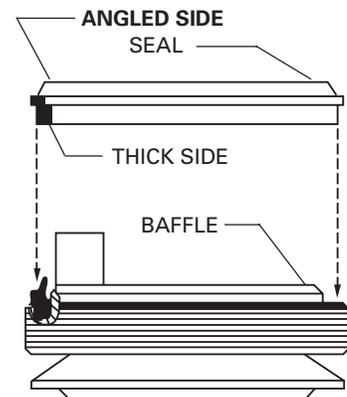
4. Assemble seal to baffle with **angled side up** as shown above. **NOTE:** The seal should be a tight fit on the baffle. If it is a loose fit on the baffle, assure that it is assembled with the angled side up.
