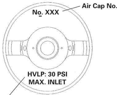
Maximum air pressure required to assure compliance of 10 PSI Max. Cap Pressure - this reading must be taken at the spray gun handle inlet fitting.
