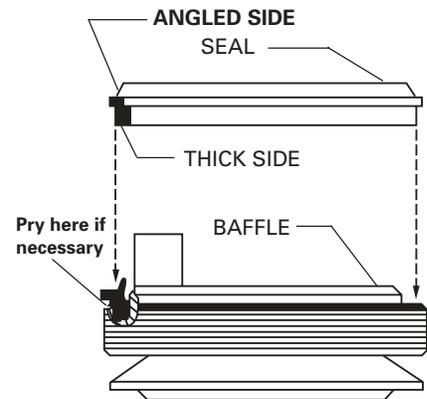
4. Assemble seal to baffle with **angled side up** as shown above. **NOTE:** The seal should be a tight fit on the baffle. If it is a loose fit on the baffle, assure that it is assembled with the angled side up.
