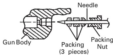
1. Remove adjusting knob and needle spring from gun.
