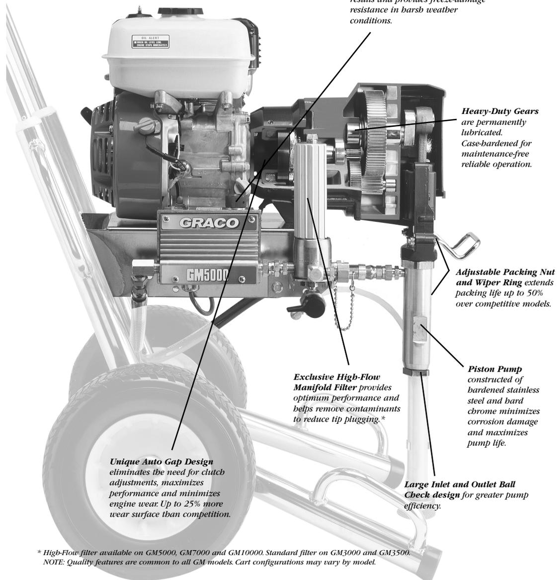
*Heavy-Duty Gears are permanently lubricated. Case-hardened for maintenance-free reliable operation.*
