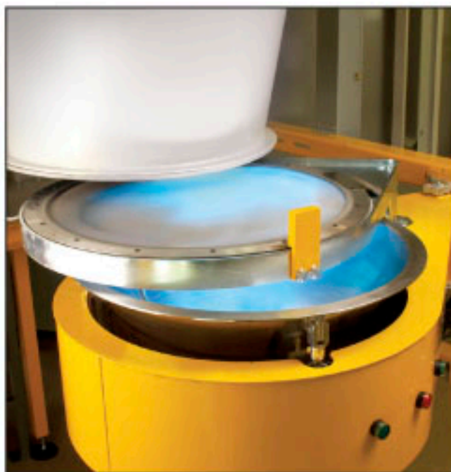
The built-in sieve in the cyclone is easy to clean during color change.
