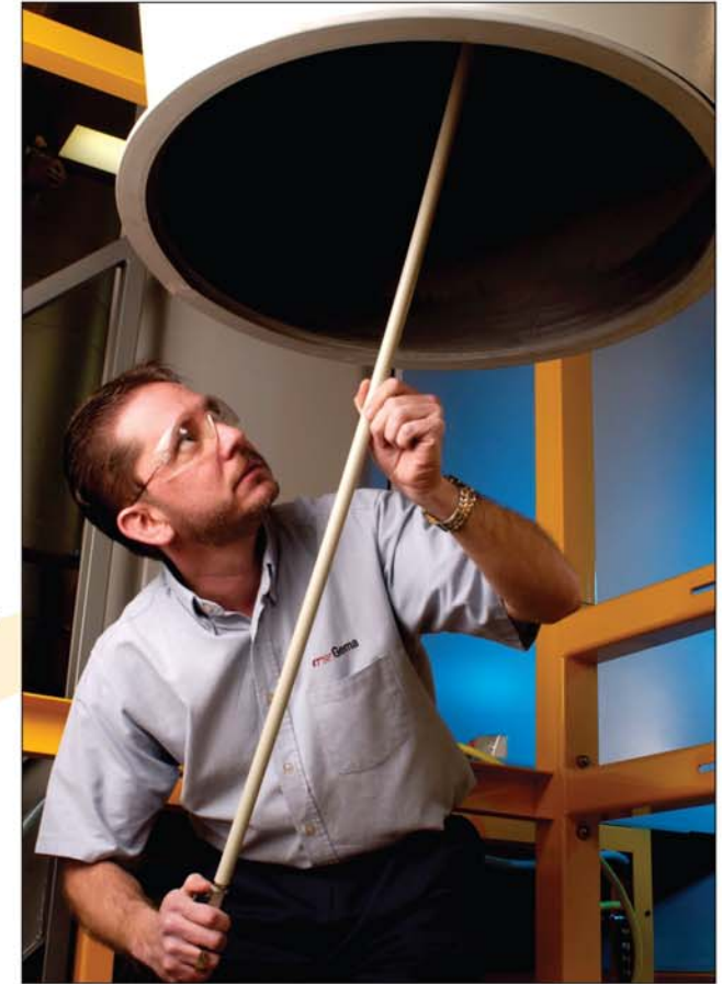
The improved cyclone is designed for optimum accessibility, making it easy to clean.
