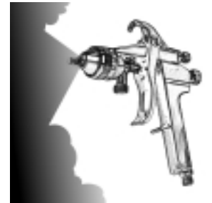
Conventional High Pressure Spray Gun Overspray
